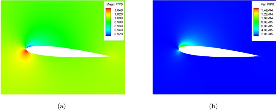
**Figure 5.** The mean(a) and the variance(b) pressure field obtained from a 4<sup>th</sup> order Probabilistic Collocation computation, with Fine<sup>TM</sup>/Hexa as deterministic solver.
